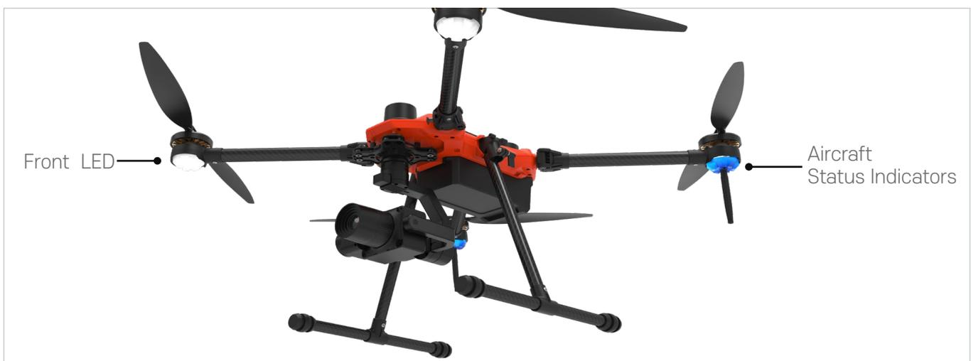
The Front LEDs show the orientation of the aircraft. The Front LEDs glow solid white when the aircraft is turned on to indicate the front (or nose) of the aircraft. The Aircraft Status Indicators communicate the system status of the flight controller. Refer to the table below for more information about the Aircraft Status Indicators.
